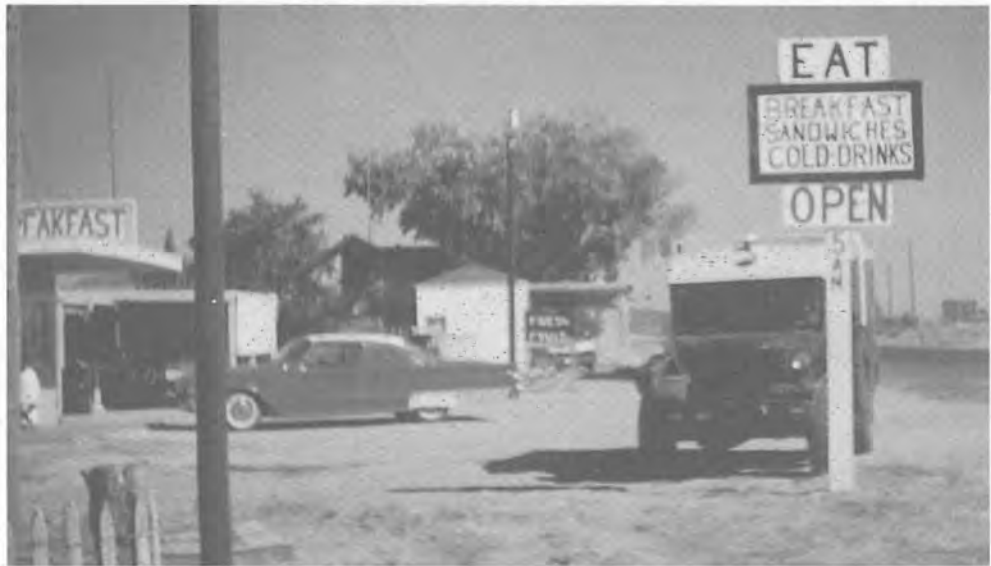
Fig. 64. Balloon Branch vehicle at roadside café. This M-43 3/4-ton field ambulance, converted by the Holloman Balloon Branch into a communications vehicle, was a common sight in the areas surrounding Roswell during the 1950s and early 1960s. (photo collection of Ole Jorgeson)
