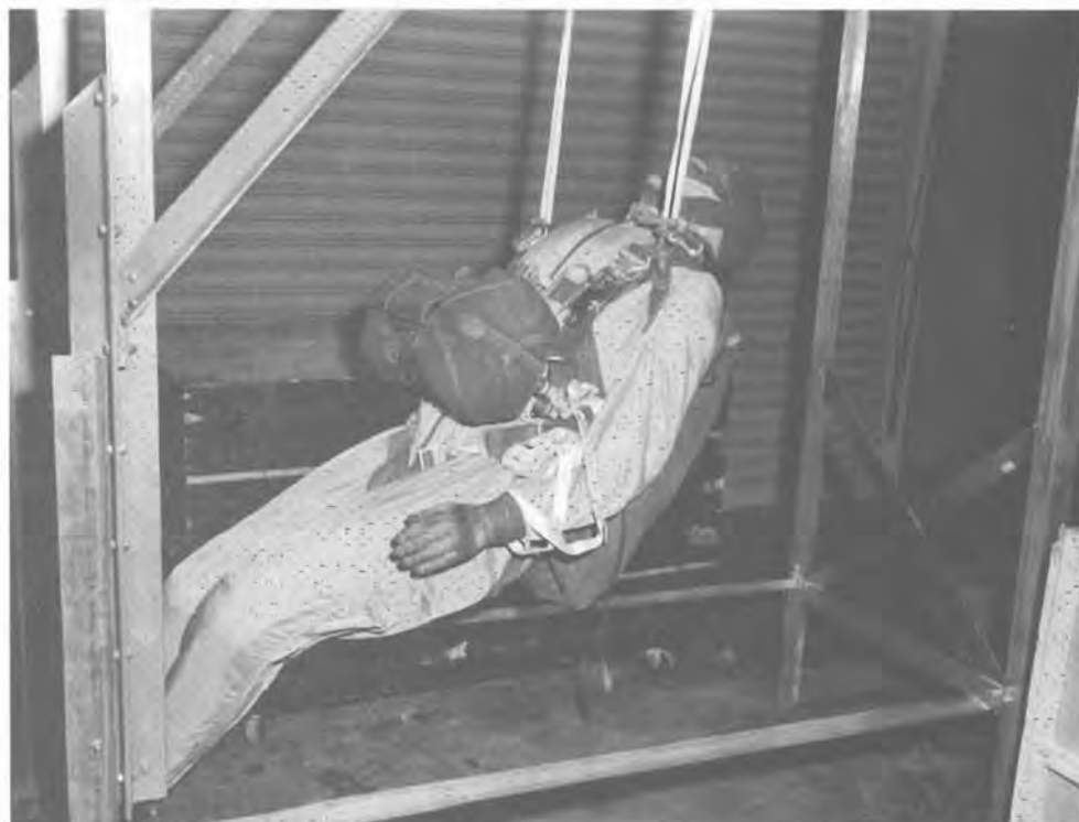
Fig. 74. “They looked like they had some sort of bandages on ‘em...over his... arm... around his midsection and partially over his shoulder”—witness description of tape and nylon webbing used to prevent arms and legs from flailing, and parachute harness that had chest and shoulder straps. Tape was also used to secure the removable back plate of the head (also see figs. 29, 30, 73,75). (U.S. Air Force photo)
