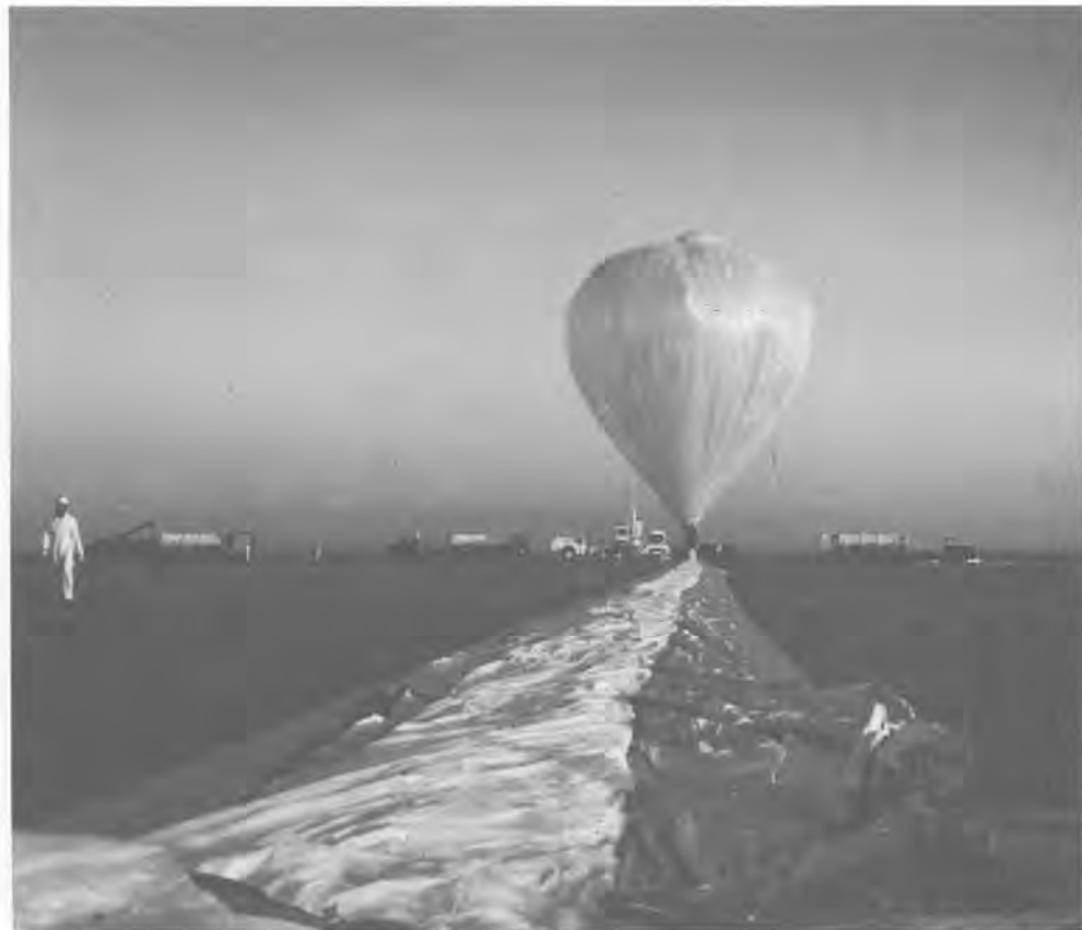
Fig. 44. Inflation of a U.S. Air Force 626 ft. long, 34.6 million cu. ft. research balloon on August 13, 1972. This balloon was launched from Roswell Industrial Air Center (formerly Roswell AAF), Roswell, N.M., to test components of the NASA VIKING space probe. (photo by Ole Jorgeson)
