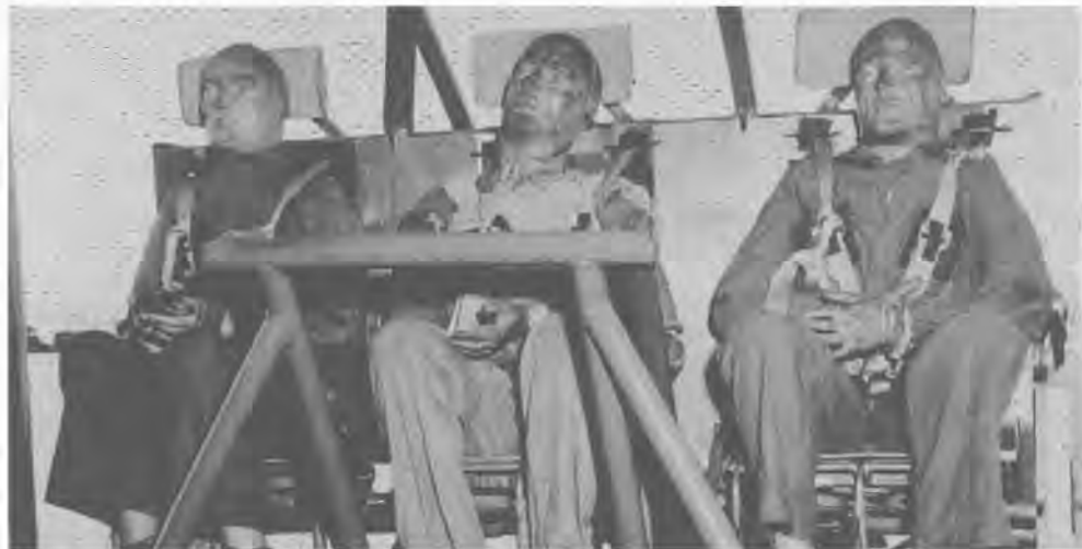
Fig. 72. “Their heads were hairless...no eyebrows, no eyelashes, no hair,” a likely description of Alderson Laboratories type anthropomorphic dummy. These Alderson dummies, of the same type used for Projects HIGH DIVE/EXCELSIOR, were used to test NASAs APOLLO spacecraft three-man couch at Holloman AFB, N.M. in 1965. (U.S. Air Force photo)
